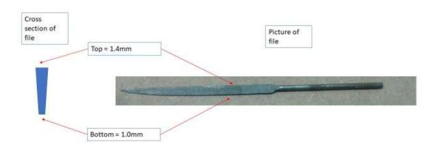
I simply run this file carefully through the check rails until the bottom edge touches the sleeper base on the point. I don't make any other changes to the point, but do check the back to back on the wheels to match the Society standards.
