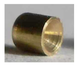
A shim of 0.5mm thickness plasticard is inserted between the wheelset and the chassis on one side to ensure that the wheelset is centred, and the bearing is inserted on the other side with tweezers:
