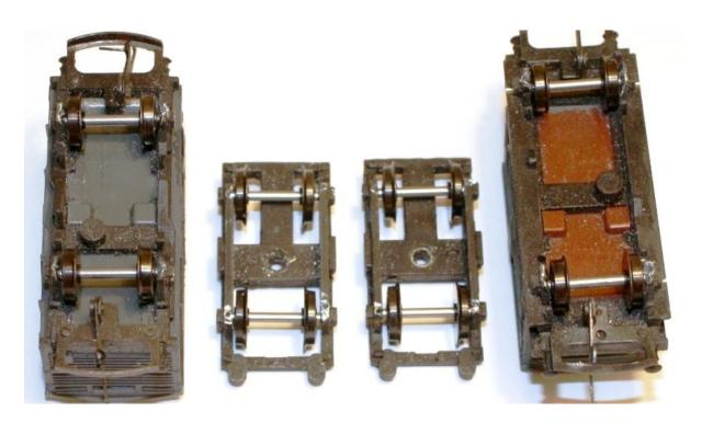
Now the 2mm diameter rimless bearings (also available from 3SMR) are inserted into the axleboxes
