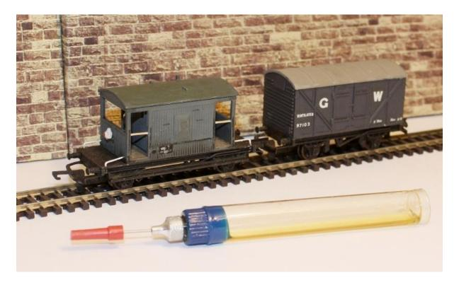
With a drop of oil into the bearings and some solid running-in there you have it: surefooted, smooth and free-running Tri-Ang rolling stock. :^)
