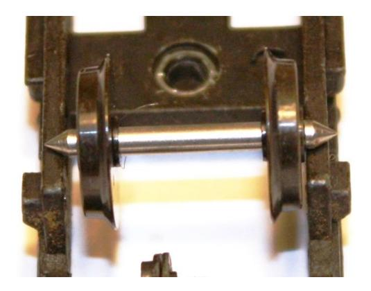
This picture demonstrates the first problem to be overcome, the axles are 20mm wide from point to point and the inside chassis frame is only 17mm, so they can't just be dropped in.
