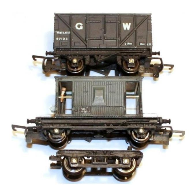
A lick of matt black paint covers the bearing ends and any scratches to the chassis
