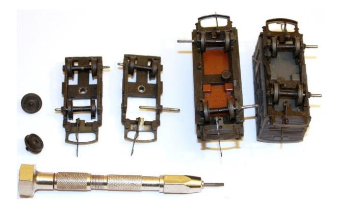
The axles are splined on one end to prevent them from falling out,
